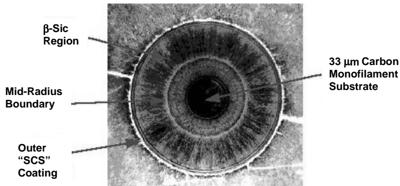
FIGURE 3.2.2.2(b) Micrograph of cross section of SCS fiber.
